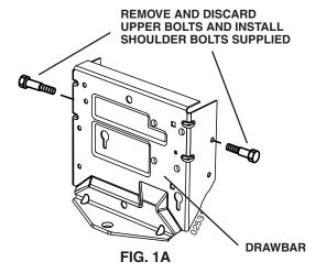
2. Install adapter to both sides of support assembly as shown.
